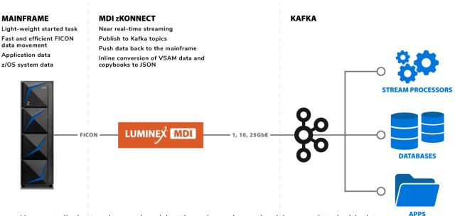
zKonnect eliminates the overhead, bottlenecks and security risks associated with data movement over mainframe-based TCP/IP, enabling more efficient and agile streaming data pipelines by using FICON.
